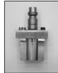
Fig. 5 The electrode of a tensile specimen
