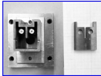
Fig. 4 The electrode of an 17 mm curved CT specimen
