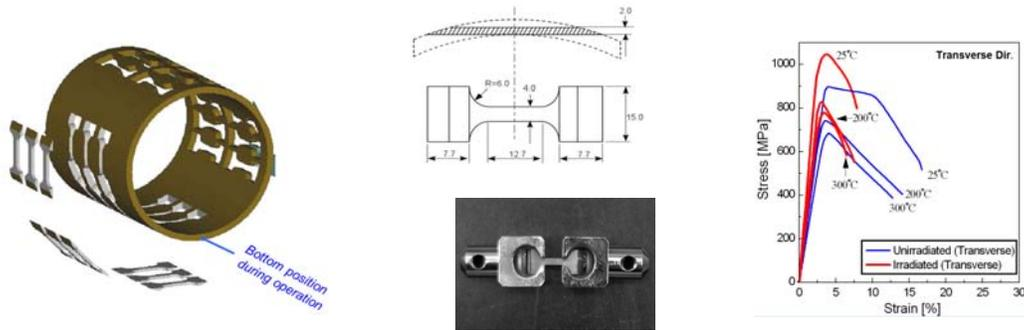
Fig.6 A cutting plan of the tensile specimen in the irradiated tube
