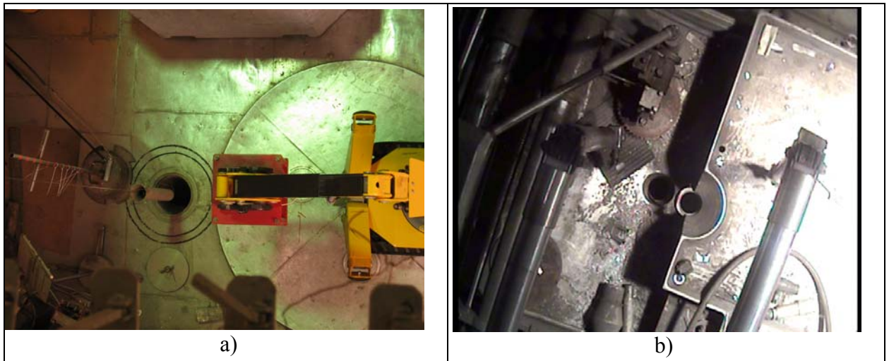
Fig. 1. a) Photo of reactor hall with top hatch of the hot sell on floor reactor. b) Photo of mechanisms for a fragmentation of investigated samples in the hot cell.
