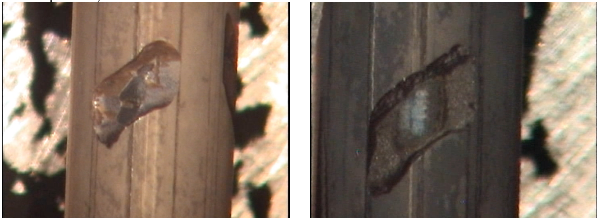
FIG. 2.2. Grid-to-rod fretting failure on several fuel rods at Temelín site.
