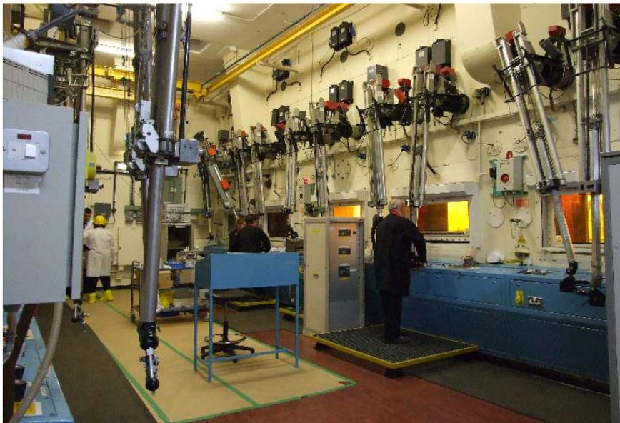
FIG. 2.2. Typical Windscale hot cell operating face.
