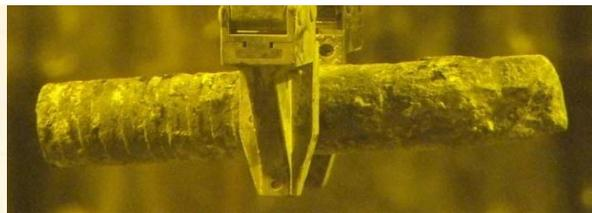
*FIG. 3.7. Cleaned uranium bar piece after removal of Magnox cladding.*
