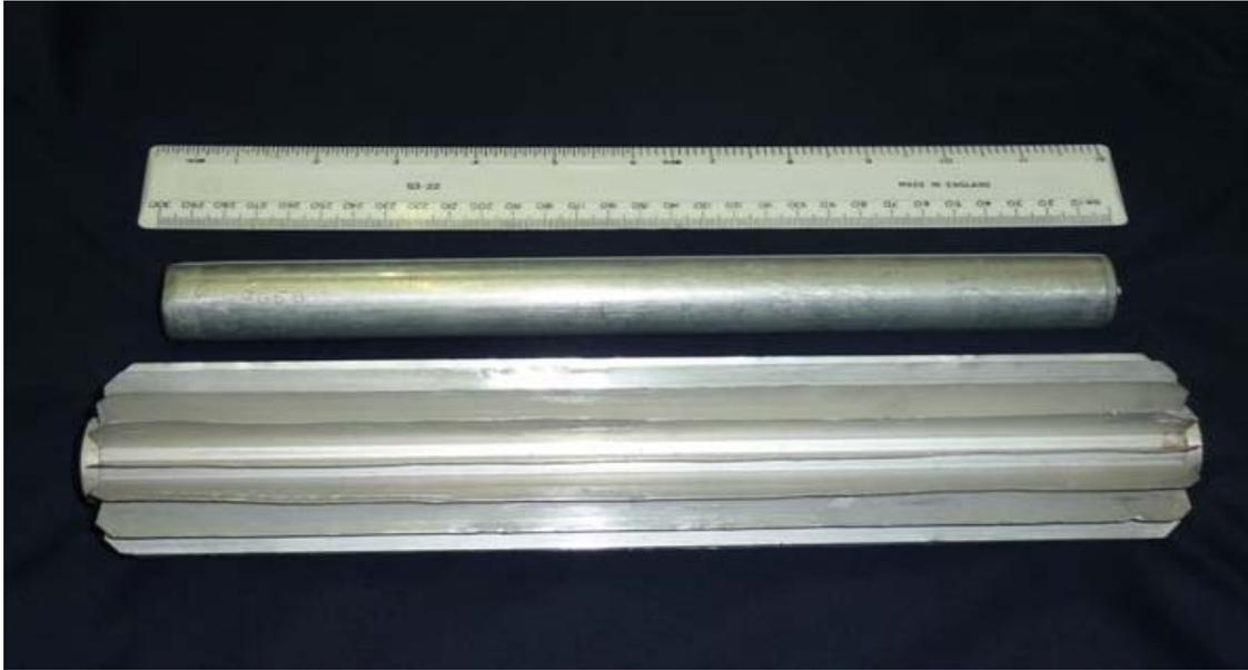
*FIG. 3.2. Pile isotope cartridge (upper) and fuel element (lower).*
