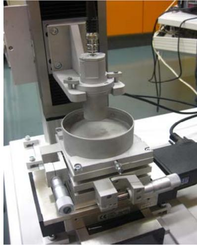
FIG. 2.2. Overview of the device showing acoustic sensors, coupling liquid holder, sample platform, translation stages.
