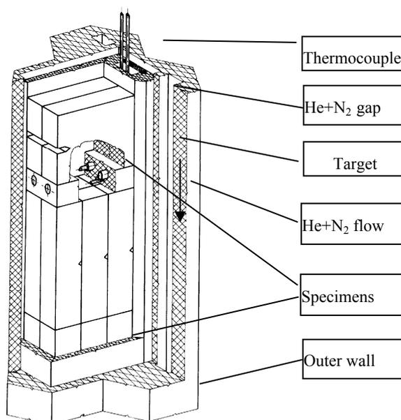
FIG. 2.1. Cross section of BAGIRA-1 irradiation rig.
