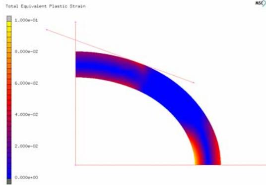
Fig. 5. Total equivalent plastic strain in ring.
