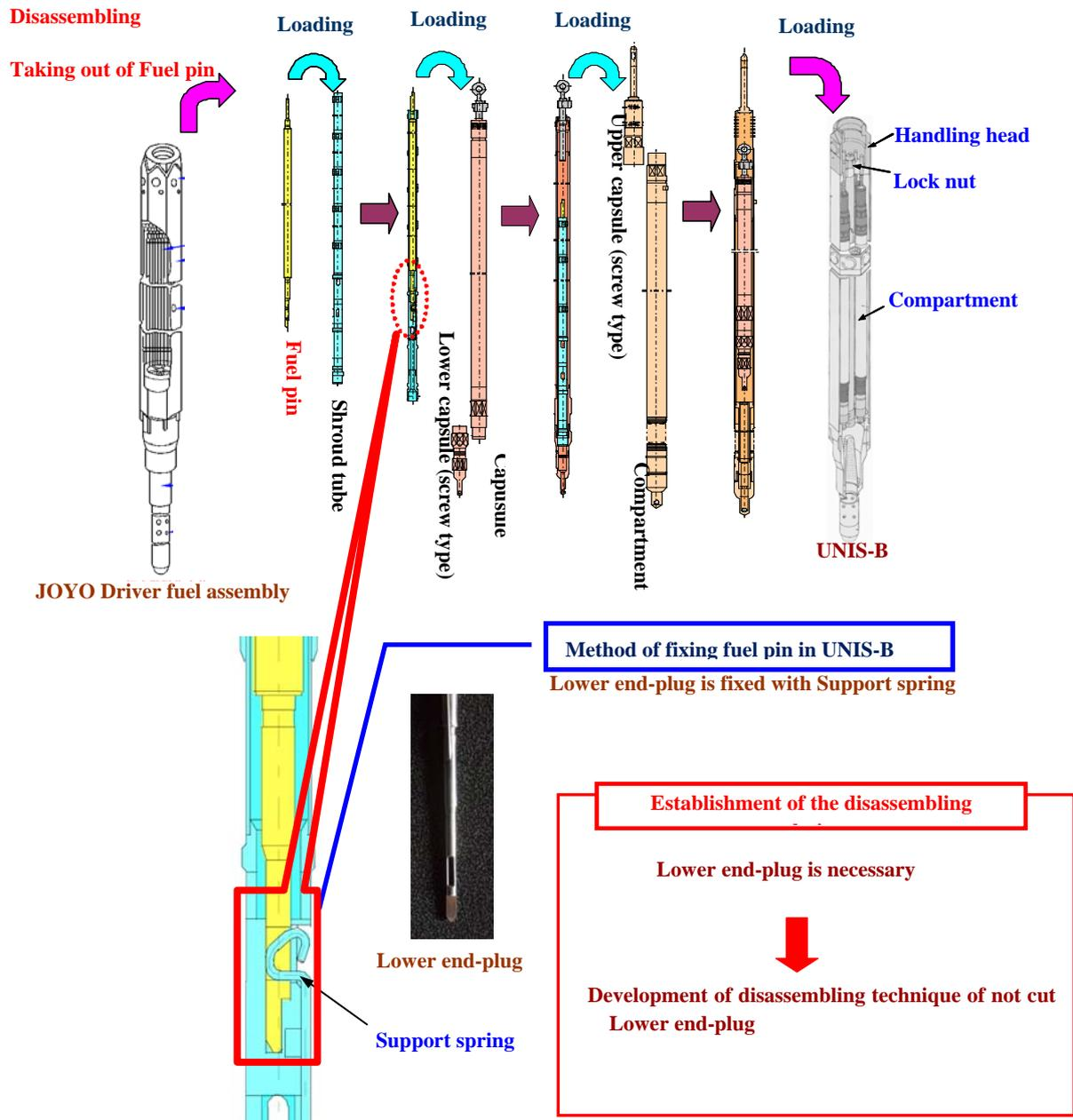
FIG. 2.2. Method for loading UNIS-B.
