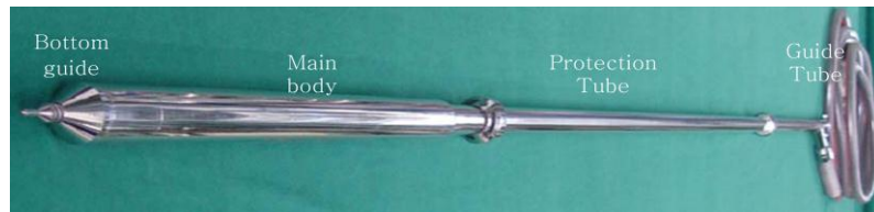
Fig. 2. Instrumented capsule for the material irradiation testing.
