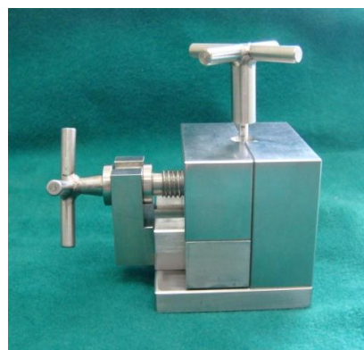
Fig. 11. Tool to dismantle a new F/M in hot cell.
