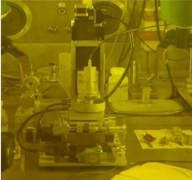
**Figure 2 : nuclear setup for acoustic microscopy in a hot cell**
