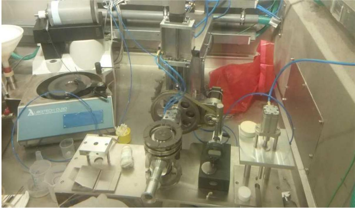
Fig. 7 Polishing equipment setup in a semi - hot cell
