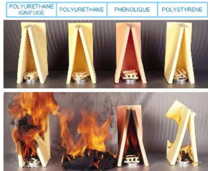
**Figure 3 – Fire test comparison between Fenosol™ phenolic foam and fireproof Polyurethane, polyurethane and polystyrene foams.**
