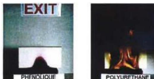
**Figure 4 – Fire Test comparison between phenolic and polyurethane foam**
