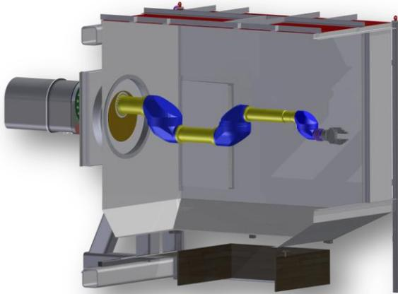
Fig. 1. 3-D Model of TELBOT installed in a box
