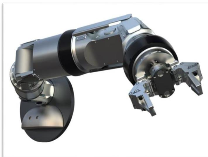
Fig. 6. Hydraulic Manipulator
