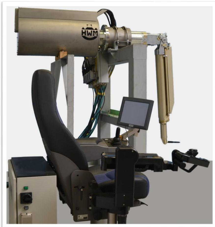
Fig. 1. Servo-Manipulator HWM A100S with drive unit on the through-wall tube and controlled by JOYARM
