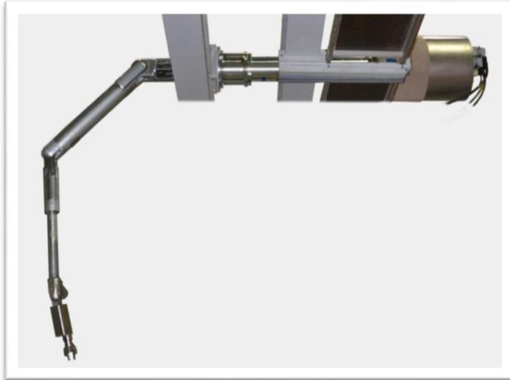
Fig. 5. Power Manipulator with standard components as 3-D Model before installed in a through-wall tube
