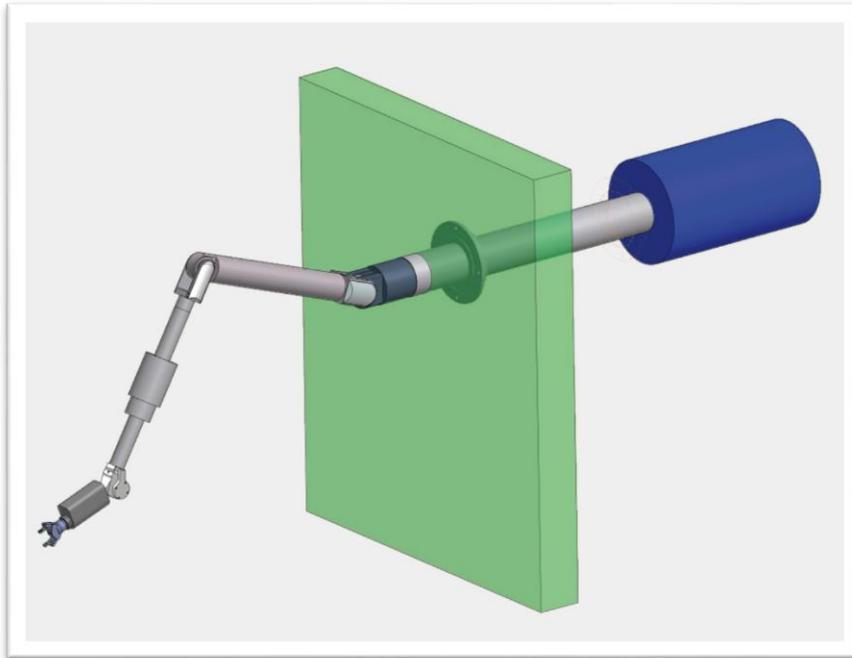
Fig. 4. 3-D Model of a power manipulator installed in a liner tube
