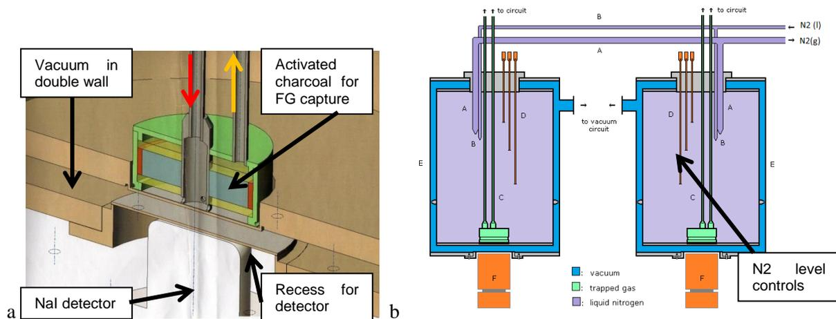
Fig. 5 a) detail of the KTG Dewar vessel with its double wall and the cold trap filter with an activated charcoal for collection of the fission gases; b) diagram of overall layout of the cold traps, their vacuum and the circulation of the liquid N<sub>2</sub> cooling system and its level controls. This ensures efficient freezing out of the fission gases on the charcoal filter for detection of the Kr-85 gamma line by NaI detectors
