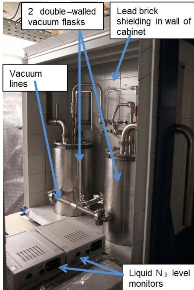
Fig. 4 photograph of the lead-lined cabinet showing the cold trap inside the lead shielding and the 2 liquid nitrogen level monitors at the front.
