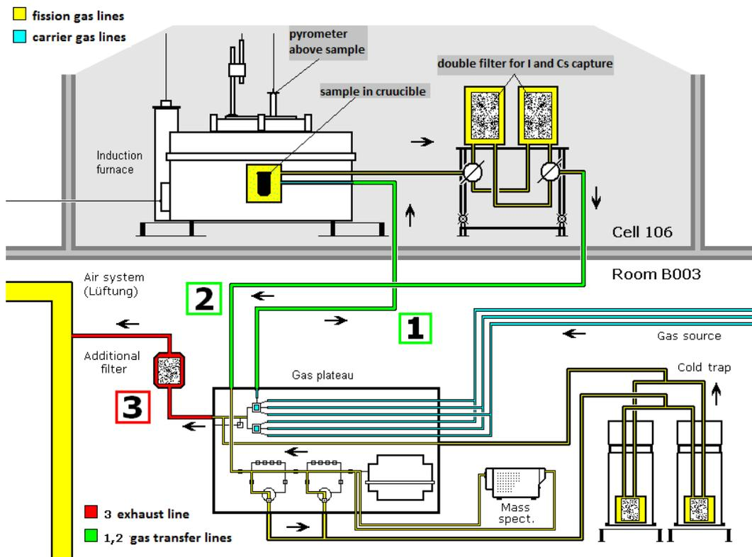
Fig. 2 Complete ITU facility for fission gas release measurements showing the gas circulation between the high temperature oven in the hot cell and the gas-mixing station attached to  $N_2$ -cooled cold traps with gamma spectrometers and mass spectrometer in the basement.
