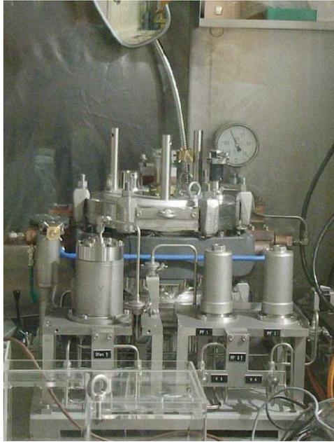
Fig. 1 High temperature furnace in the hot cell during installation in the hot cell
