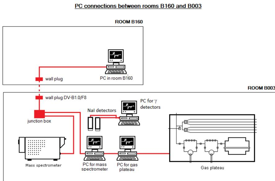
Fig. 6 showing the connections between the computers in the fission gas measuring system.
