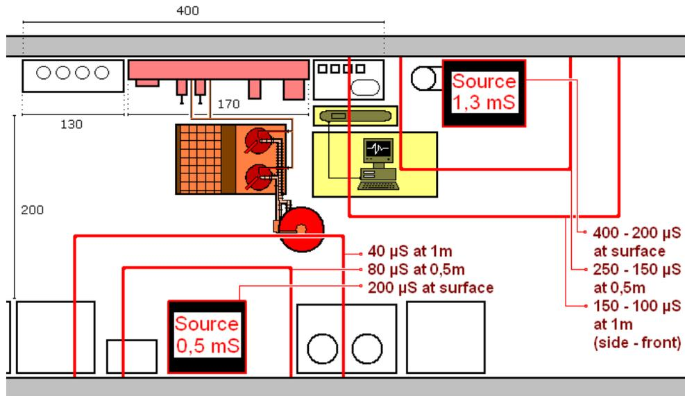
Fig. 7 Diagram of the lowered dose rates in the basement below the Hot Cells at points near the gas-mixing tableau, the cold traps and the PC desk of the FG facility.
