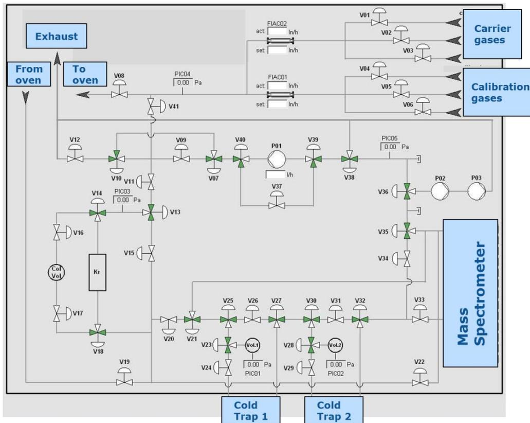
Fig 3 Flow scheme for the Gas-mixing facility as shown on the Software for mixing system monitoring
