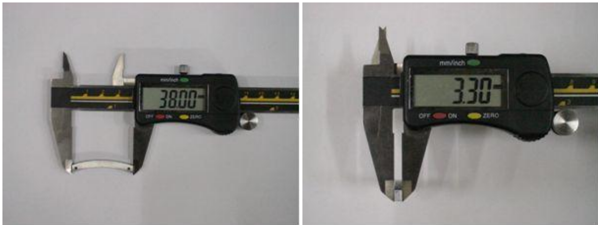
Fig. 5.2 C-shaped sample measurement after machining
