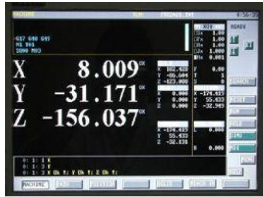
Fig. 3.4 Drill no. 1 measurement using the TS27R instrument
