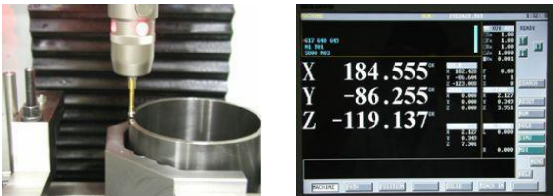
Fig. 3.2 Pressure tube measurement using the Point Finder
