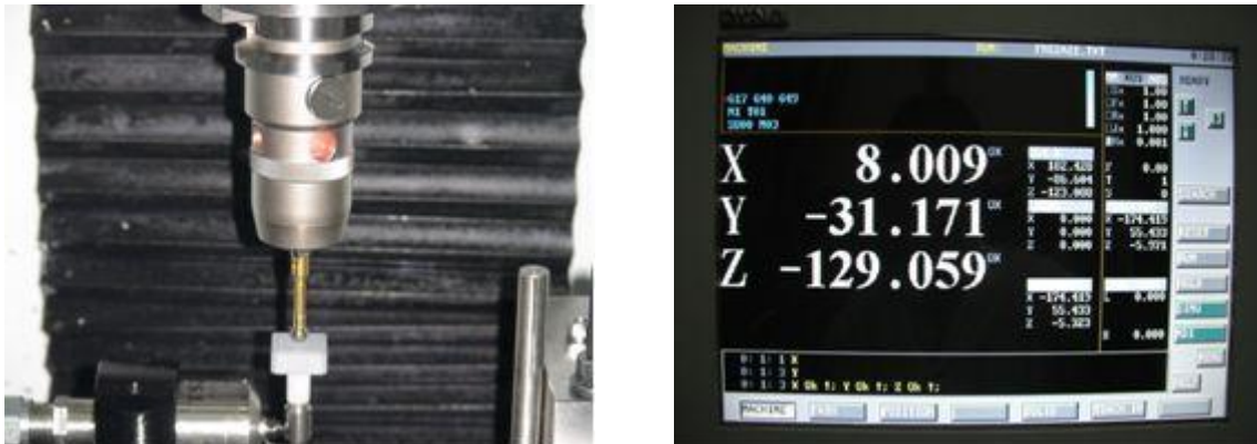
Fig. 3.1 Point Finder measurement using the TS27R instrument
