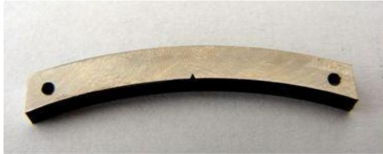
Fig. 5.1 C-shaped sample out of irradiated CANDU pressure tub for KIH mechanical test
