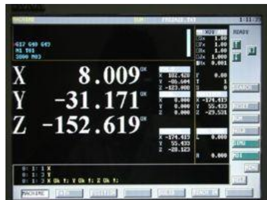
Fig. 3.6 Mill no. 3 measurement using the TS27R instrument
