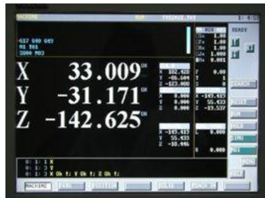
Fig. 3.5 Mill no. 2 measurement using the TS27R instrument
