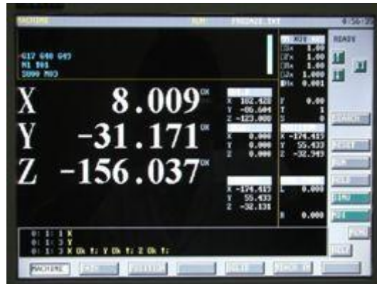
Fig. 2.1 Machine Coordination Display
