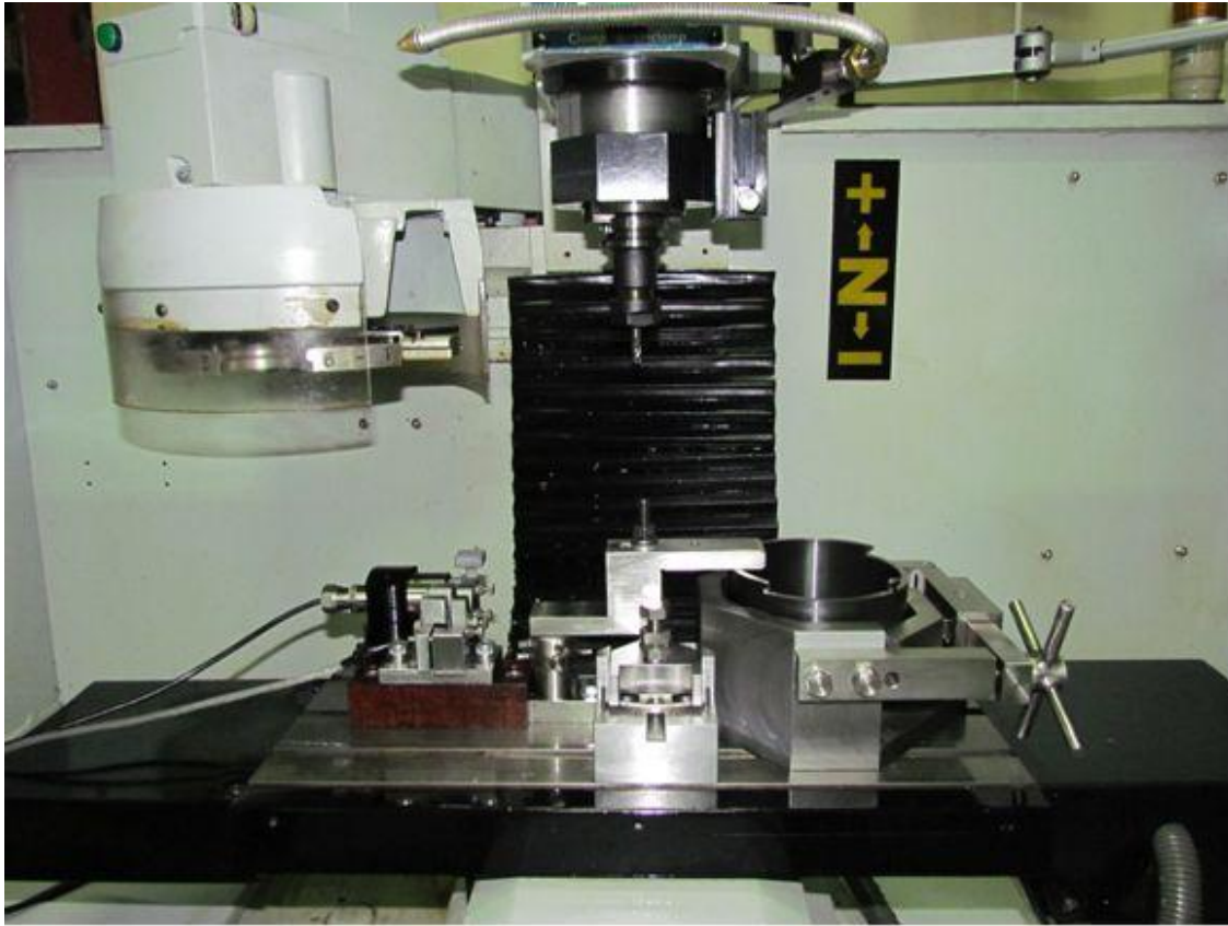
Fig. 2.4 DM 1007 Numerically Controlled Milling Machine – Overview of the working table with all devices installed
