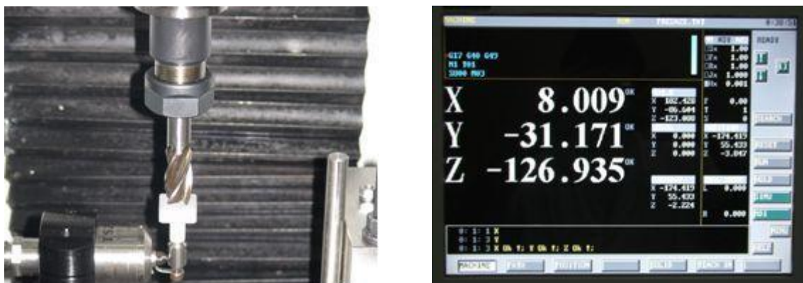
Fig. 3.3 Mill no. 1 measurement using the TS27R instrument
