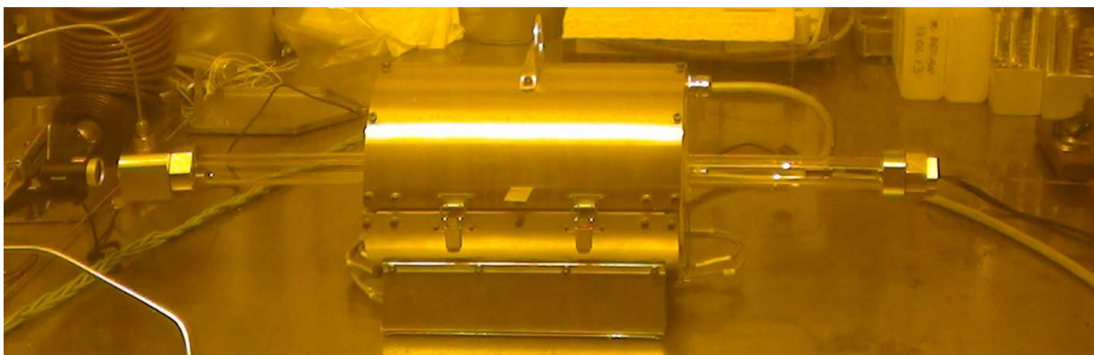
Figure 1 Furnace used for fuel heating tests installed in hot cell. Air atmosphere setup (top) and inert gas setup (bottom). The camera is visible to the left of the quartz tube.
