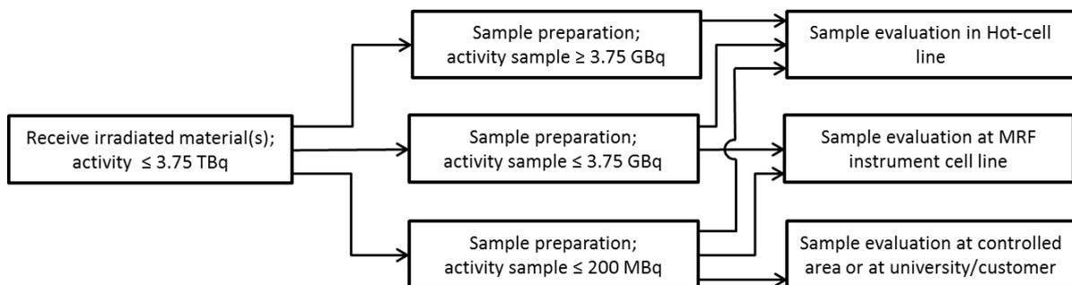
**Figure 3 Overview of sample preparation and evaluation regime in the UKAEA-MRF (activities based on  $\text{Co}^{60}$  or  $\text{Co}^{60}$  equivalent)**
