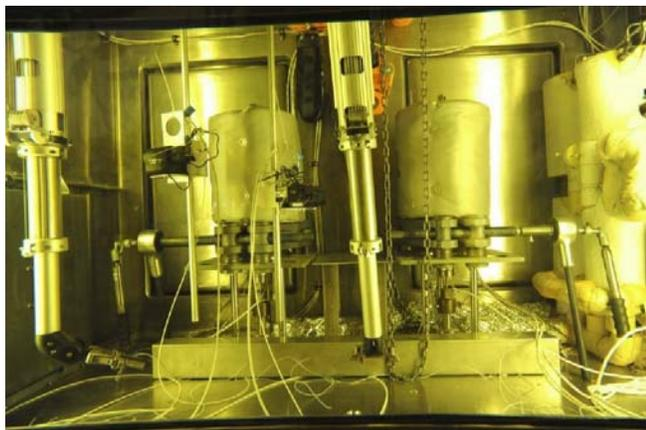
Figure 2. View of the test cell showing the two autoclaves used for IASCC testing at INL.
