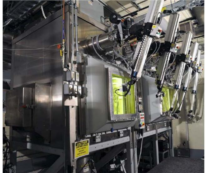
Figure 1. Overview of the test cells for IASCC testing and scanning electron microscope characterization at INL.
