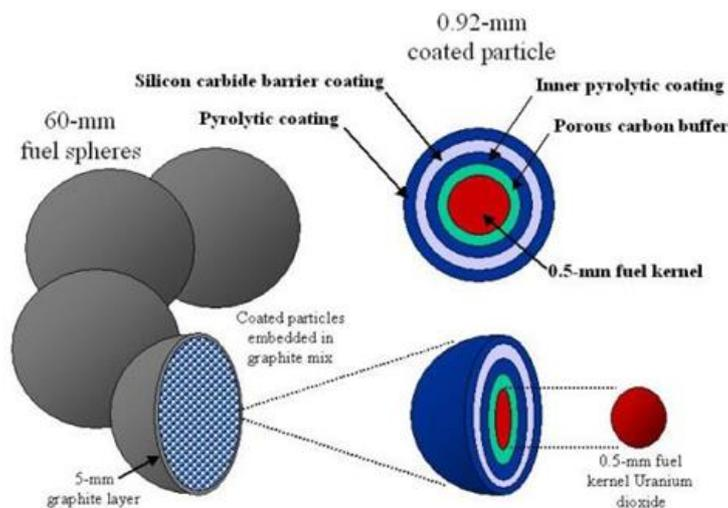
Figure 1 Structure of Spherical Fuel Element and TRISO Coated Fuel Particles
