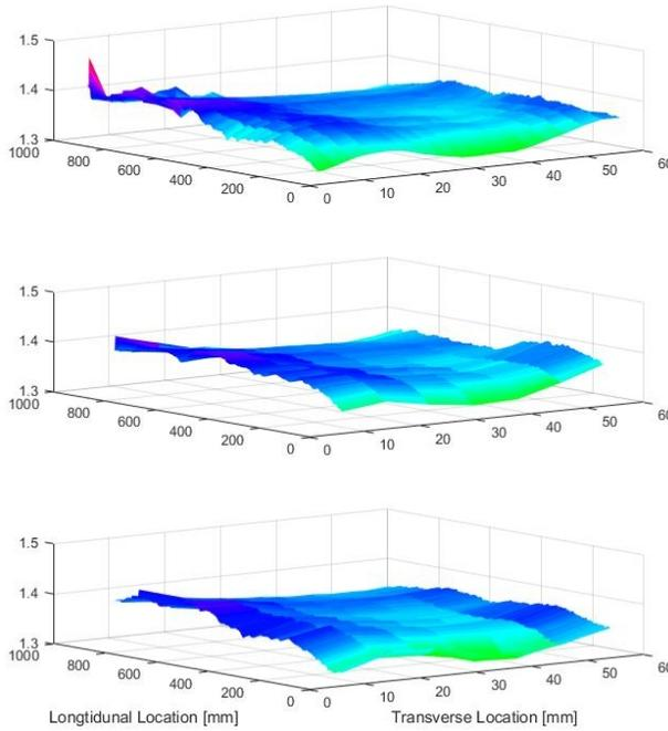
Figure 5: Surface Plot of AFIP-7 Plate 4 Repeated Scans. (Top, Scan 1; Middle, Scan 2; Bottom, Scan 3)
