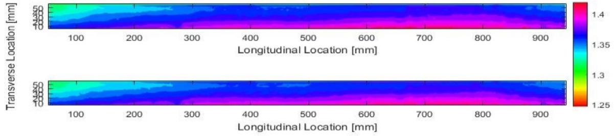
Figure 7: AFIP-7 Plate 1 Repeated Corrected thickness of Scan 1 (Top) and Scan 2(bottom)
