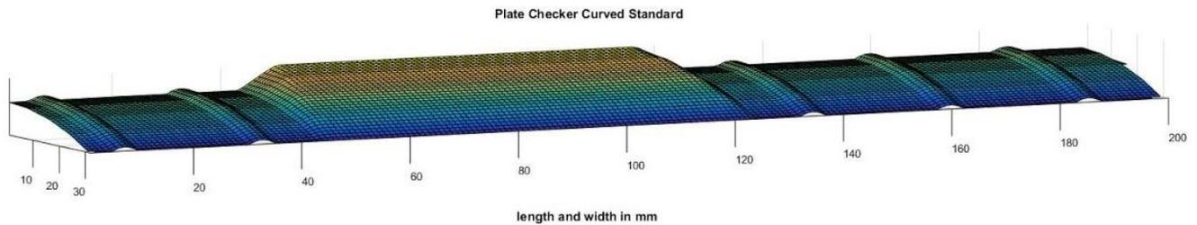
Figure 3: Curved plate standard results surface profile
