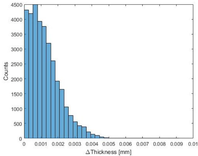
Figure 9: Thickness Variation between Plate 1 Scan 1 and Scan 2
