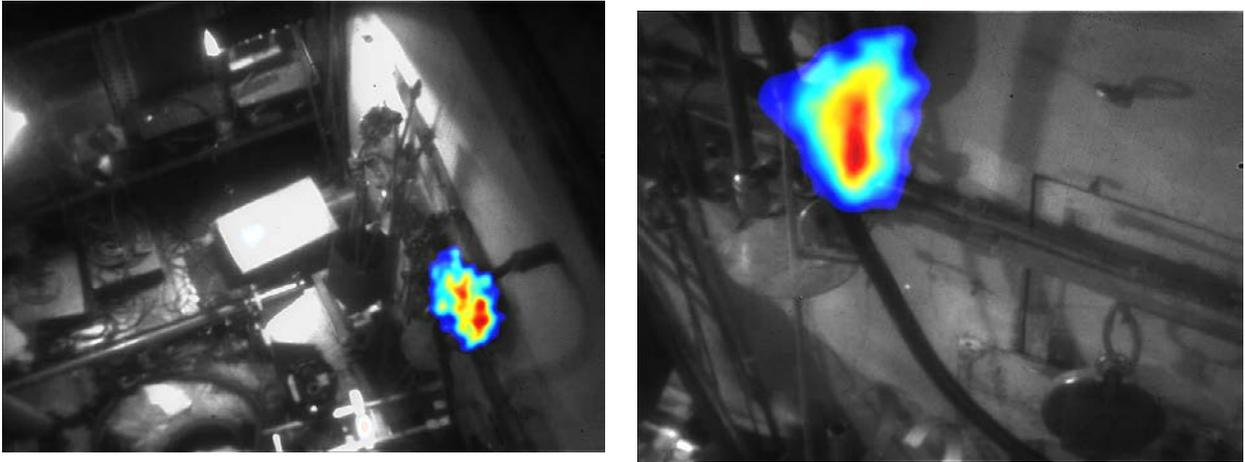
**Figure 5 Combined visible/gamma images of the hot spot detected in Hot Cell #3**
