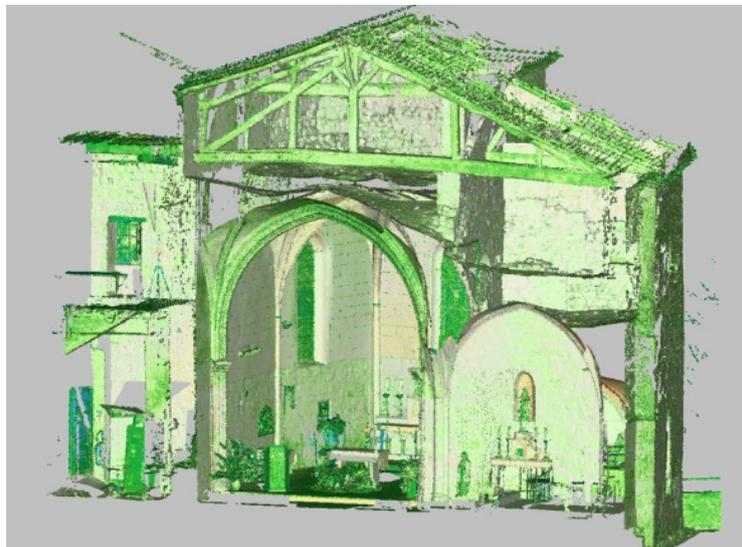
**Figure 6 : Sample scan of the inside of a church**
