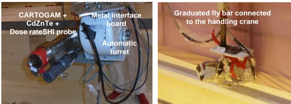
**Figure 3 : System used for the radiological investigation of the LECA Hot Cell #3**
