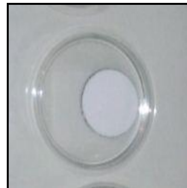
Fig. 6. The filter fastened on a stainless steel disk (Alpha source)
