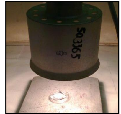
Fig. 5. Filter's dry under the UV lamp
