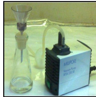
Fig. 4. Gelman filtration system
