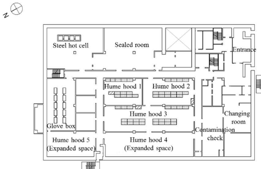
Fig. 4. Schematic layout of Laboratory-1 (Second floor plan).
