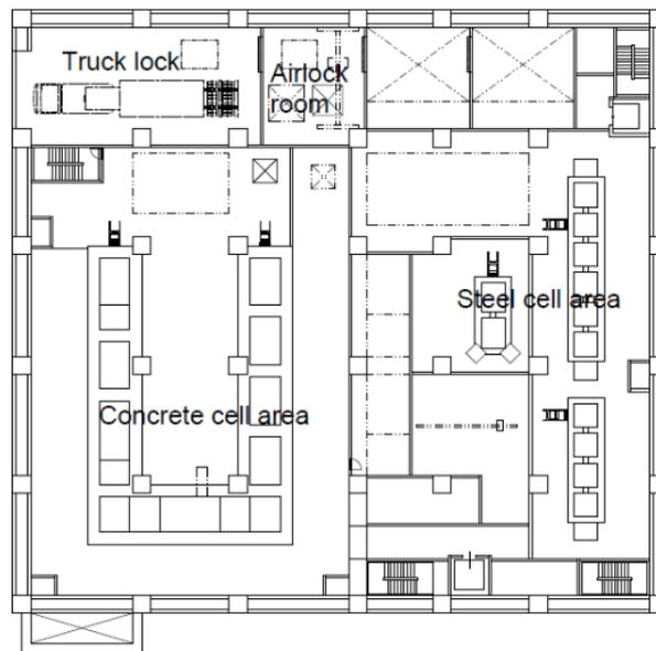
Fig. 5. Schematic layout of Laboratory-2 (First floor plan).
