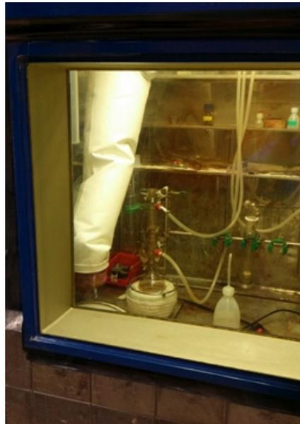
Figure 5: Active shielded dissolution box
