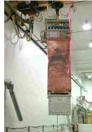
Target module transported with remote handling crane between target station and hot cell
