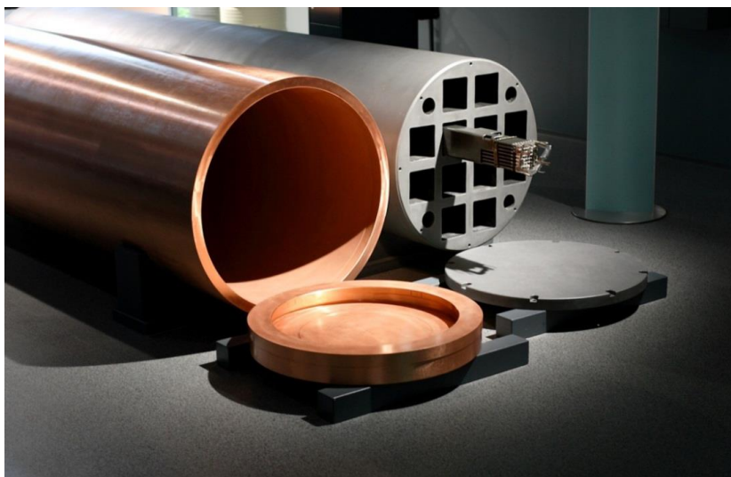
Figure 78: The spent nuclear fuel is packed into the copper-steel canister, where the steel insert has positions for the fuel assemblies and the copper shell protects the fuel from the corrosion.
