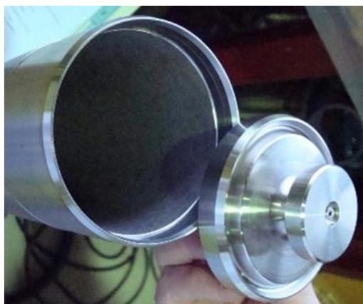
Figure 74: Stainless steel primary canister
