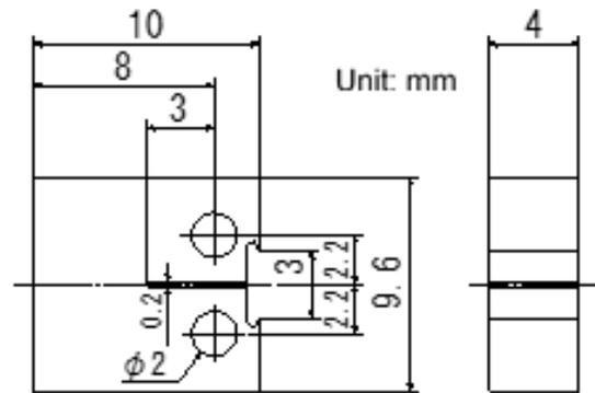
**Figure 33:** Geometry and dimensions of Mini-C(T) specimen.
