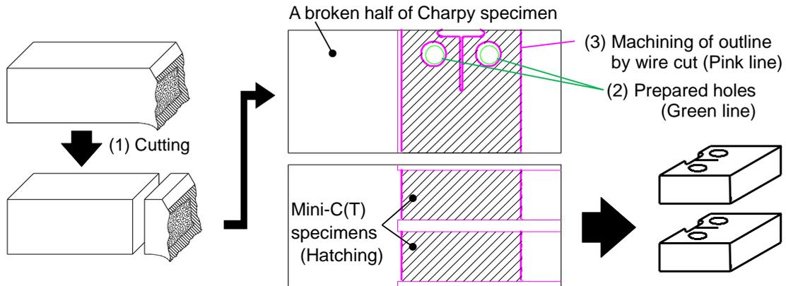
Figure 35: Image of machining process for Mini-C(T) specimens.
