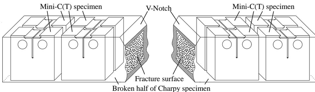
**Figure 34:** Orientation of Mini-C(T) specimens machined from broken halves of Charpy specimen.
