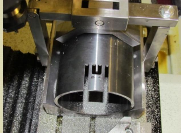
Figure 4. Separation of the CT sample from the pressure tube fragment
