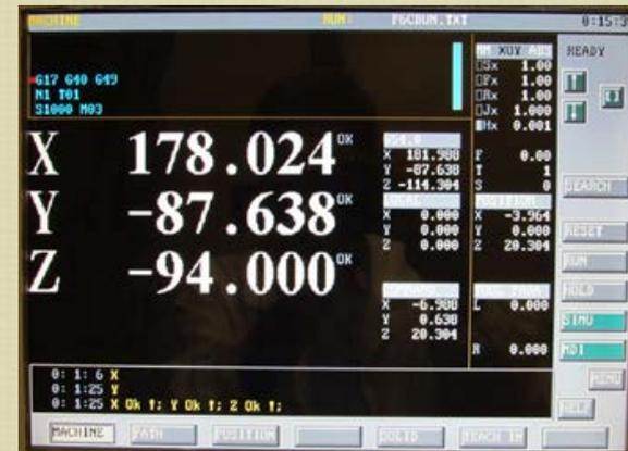
Figure 3. Measurement of the pressure tube coordinates using the „Point Finder”
