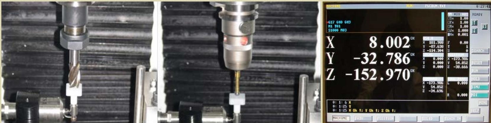
Figure 2. Tools measurement using the TS27R instrument
