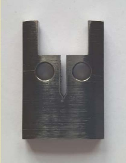
Figure 7. CT sample manufactured out of non-irradiated CANDU pressure tube
