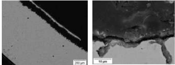
Fig. 2 SEM micrographs indicating chemical interaction between FeB and SS 304L clad
