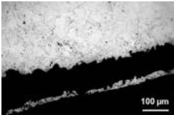
Fig. 1 Microstructure of the SS 304 L clad showing the clad attack clad
