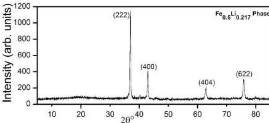
Fig. 3 XRD pattern at the interface region showing the  $\text{Fe}_{0.5}\text{Li}_{0.217}$  interaction phase.
