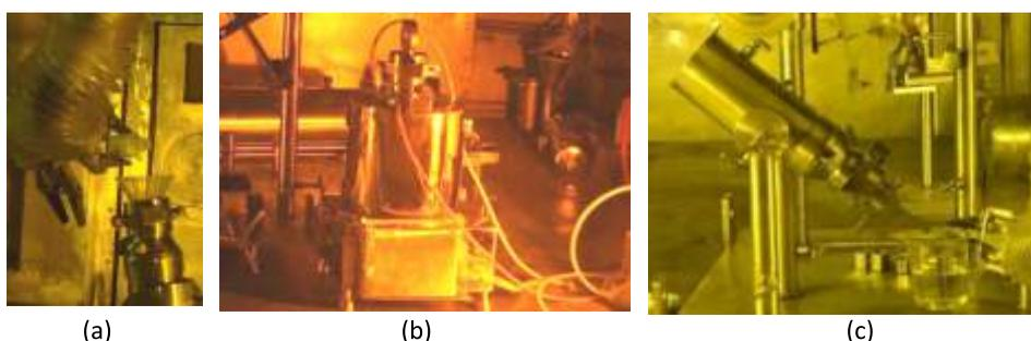
Figure 6 (a) Transfer of pellets and acid for dissolution (b) Heating unit (c) Transfer of dissolver solution
