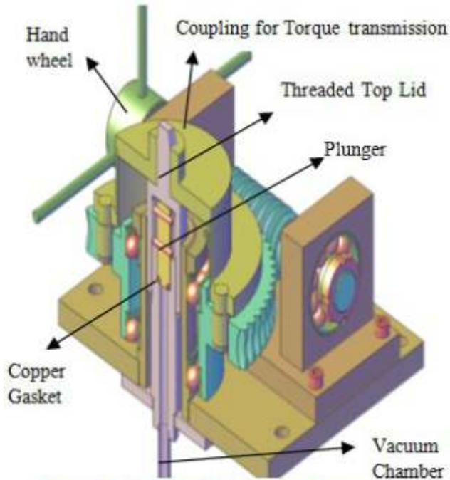
Figure 2. Remote Sealing Arrangement
