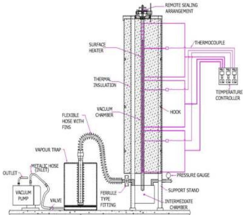
Figure 1 : Vacuum Distillation System
