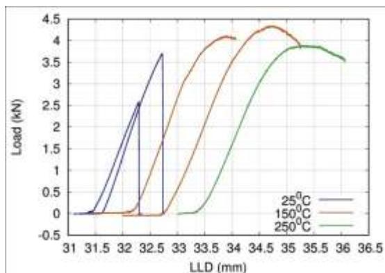
Figure 1. Load vs load line displacement (LLD) obtained for fracture toughness test specimens at different temperatures.
