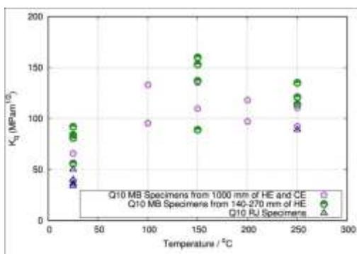
Figure 2: Fracture toughness of Q10 pressure tube main body (MB) and rolled joint (RJ) region after 15.3 HOY.
