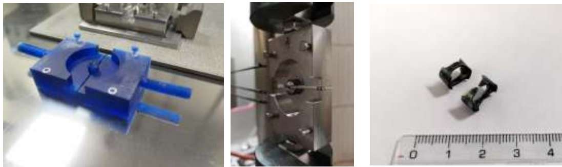
Figure 2. The holder design evolution (left and middle), specimens before and after the test (right)
