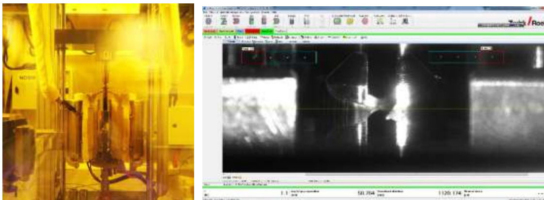
Figure 3. Creep machine inside the hotcell (left), specimen image from video/laser extensometer (right)
