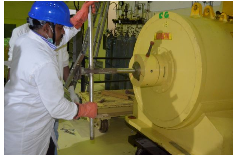
Y 2 O 3 pellets were posting in to Hot cell through EXTP.
