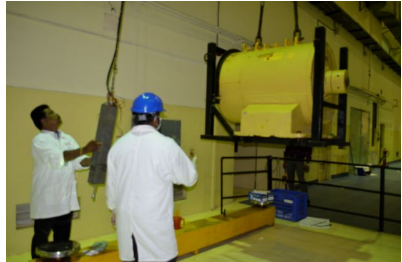
Unloading the lead cask
