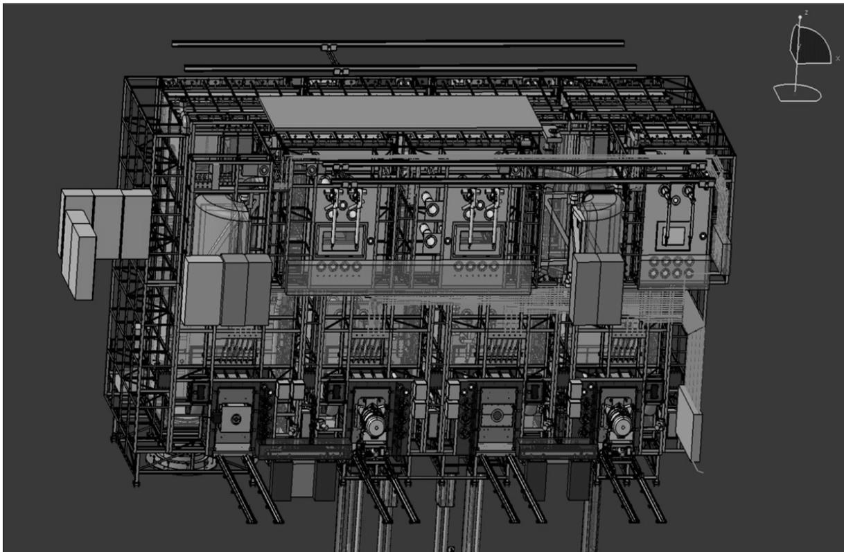
Fig 2. General view of the hot cells complex in CATIA. Large cells back zone is visible at the bottom, small cells front zone at the top.
