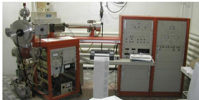
*Thermal Ionization Mass Spectrometer (TIMS)*
