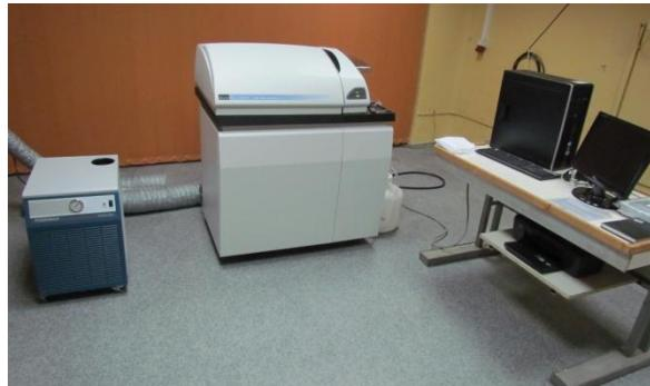
*ELAN DRC-e Quadrupole ICP-MS*
