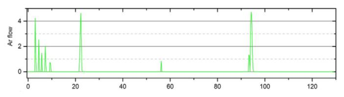
**Correct: Smaller flow** than flowmeter can detect
