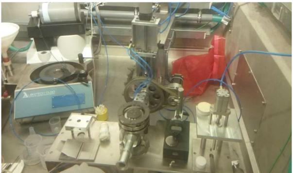
Fig. 7 Polishing equipment setup in a semi - hot cell
