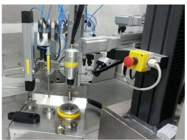
Fig. 8 The equipment for assembly of the specimens testing fixtures and manipulation of the single SPT specimens in semi-hot cell
