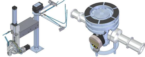
Fig. 6 Scheme of the robotic arm and JIG
