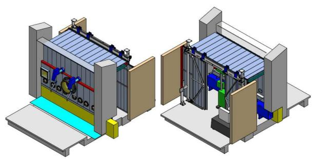
Fig. 1 Scheme of refurbishment of semi-hot cells at UJV Rez, a. s
