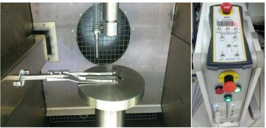
Fig. 9 Device for positioning of the tesing the samples in thermal chamber
