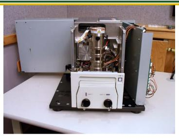
NEOSCOPE: bench top SEM with most electronic is located outside the cell
