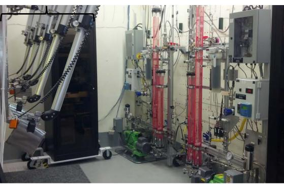
Two independent refreshed testing loops able to maintain BWR or PWR water chemistry:
