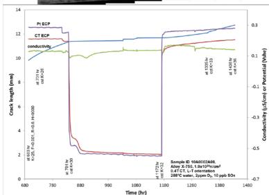
Example of crack length and water chemistry as a function of time
