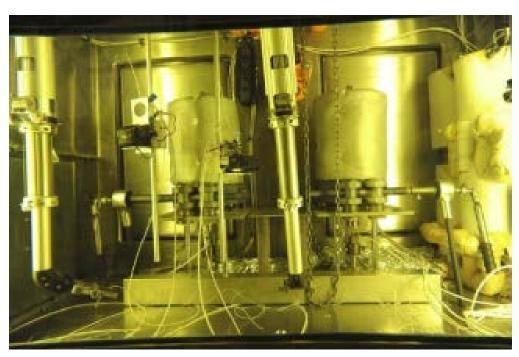
**Two** autoclaves rated for BWR and PWR testing conditions.
