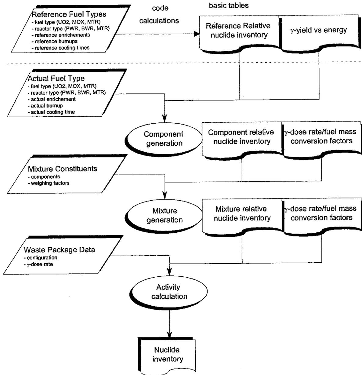
Fig. 4 : Flow-sheet of the waste characterisation module
