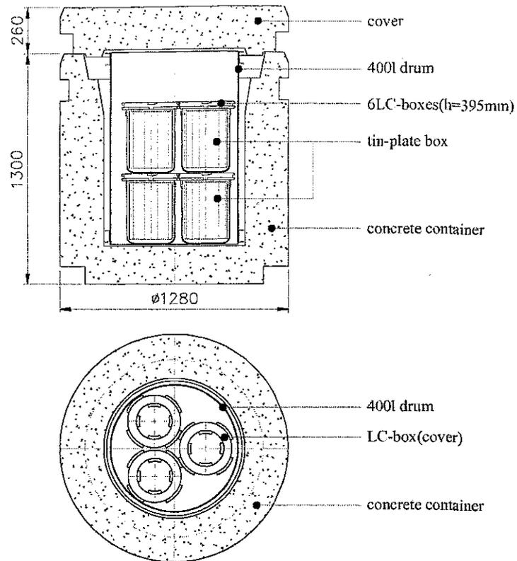
Fig. 2 : medium-level waste packaging in a standard BPIII concrete container
