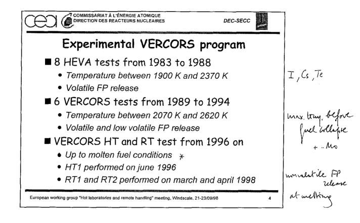
The experimental program began in 1983 with the HEVA program. **8 HEVA tests** were performed in this range of temperature around 2000 K and slightly above. The most important results were obtained for volatile FP, iodine, caesium and tellurium.
