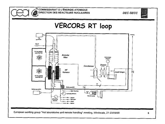
The RT version of the loop is more compact. The furnace is similar than the HT furnace, but it is more easily remote handling ; so it enables to increase the frequency of the tests. In this configuration, all FP and transuranic elements are trapped as near as possible from the emission point in a total filter. The release quantification of transuranic elements and pure  $\beta$  FP is obtained by post test chemical analyses.
