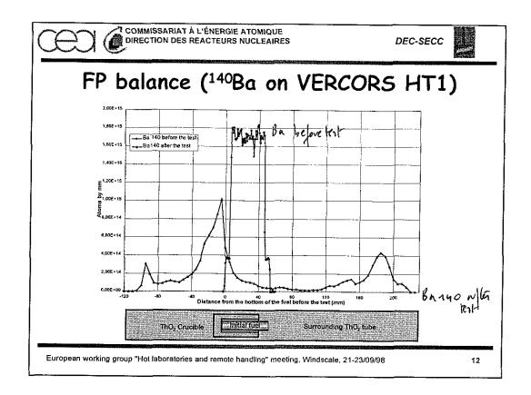
This graph illustrates, for VERCORS HT1 test, the distribution of <sup>140</sup>Ba inside the fuel sample before the test, and along the furnace after the test :
