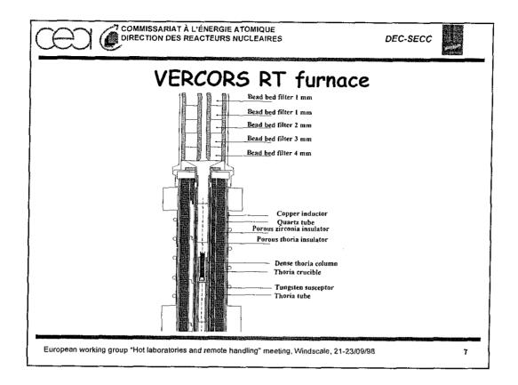
This is a zoom of the VERCORS RT furnace. The **fuel** is constituted of three pellets of enriched  $UO_2$  in their original cladding irradiated in a PWR reactor. Two half pellets of depleted  $UO_2$  are placed on each side of the test sample. For most tests, this total sample is irradiated again during one week at low power in an experimental reactor just before the test in order to recreate the short half-life FP.
