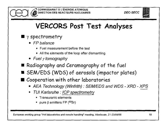
Several complementary techniques are used to quantify the release of FP and transuranic elements.
