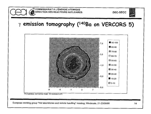
Sometimes, we perform gamma emission tomography of the fuel sample after the test. This graph gives you the radial distribution of <sup>140</sup>Ba in VERCORS 5 test, which reveals two concentric zones :
