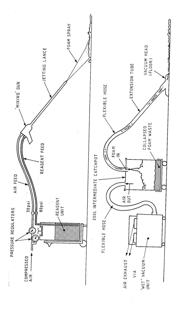
FIG. 2. FOAMING AND COLLECTION EQUIPMENT
