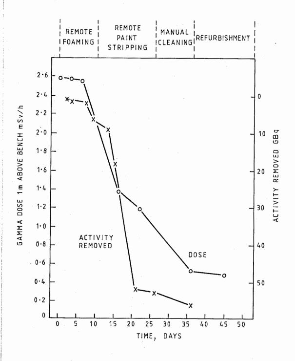
FIG. 3. ACTIVITY REMOVED AND IN-CAVE DOSE MEASUREMENTS
