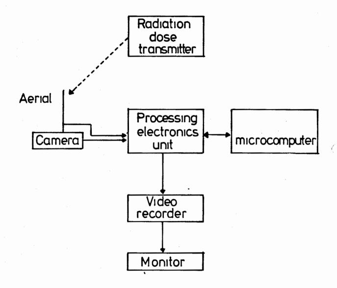
Figure 1. Lay out of the Simvidose equipment
